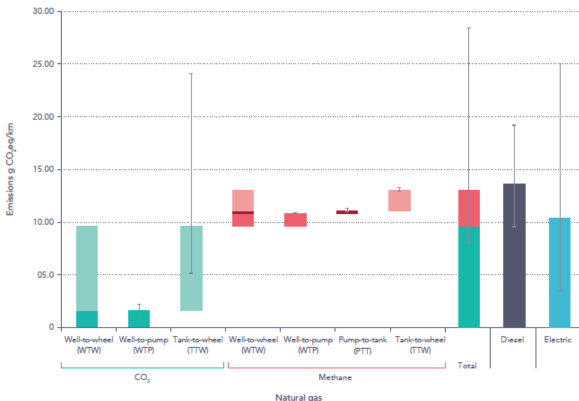
Figure 5: Emissions from the well-to-wheel life cycle of average LNG trucks for alternative fuels
